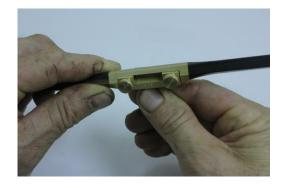
• When in position, tighten the lever cap bolts so the blade is secure.
