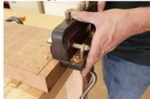
• The blade pitch in this plane will minimise tear-out, but should you encounter this, set your blade finer for a better result. If you still have tear-out you can remove the fence and run the left-hand side of the plane in your formed rebate going with the grain. Be aware you have to manually gauge the depth of the rebate.
