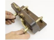
Next set the nicker blade to just below the sole of the plane. For soft wood you can go slightly deeper than you would for hardwood.
