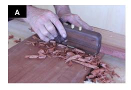
The blade depth of cut should be set so the wood is removed quickly but also ensuring the plane isn't difficult to push, otherwise the accuracy of the dado will be lost.
