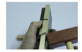
To remove the blade, simply tap the brass abutment in front of the blade, the wedge will loosen so you can remove the blade from the bottom of the plane.
