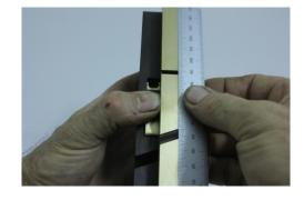
Using a small ruler, check the alignment of the nicker and the edge of the blade. Tap the blade one way or the other if required.
